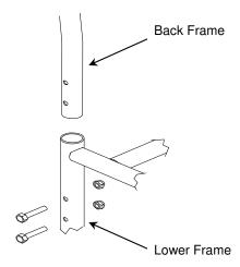
**Back Assembly-** Insert back assembly into lower frame and line up the two holes in back assembly with two holes in the lower frame. Insert bolt through hole and install nut. Repeat alignment on other side and install the other three bolts and nuts. Tighten all bolts and nuts until snug.
