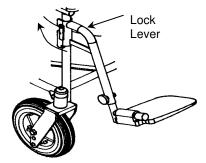
**8" Casters-** Adjust wheels that are loose and casters that flutter. The 8" wheel is secured to the caster fork by an axle bolt and nut. To adjust, rotate bolt and lock with locknut. The wheel should be snug but free spinning.
